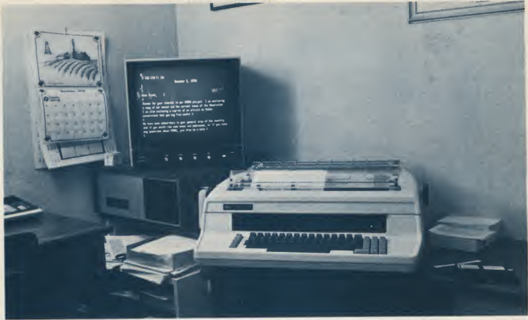
The North Star Horizon II computer, the 17 inch monitor and the NEC Spinwriter. They are mounted on a custom desk with the Spinwriter set at a 30° angle for easier viewing of the monitor.
